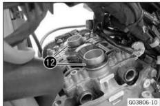
Remove spark plug shaft inserts
