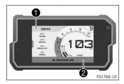
Warnings appear on the top and/or bottom edge of the display; these are marked yellow or red depending on their relevance. Yellow warnings indicate errors or information which require prompt intervention or an adjustment to the riding style. Red warnings indicate errors or information which require immediate intervention.
