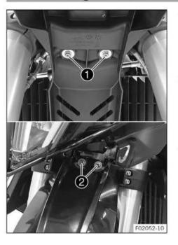
Position the front fender. Mount screws 1, but do not tighten yet.
