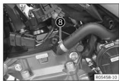
Remove hose clamp 8 and pull off the vent hose.
