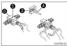
Mount press drift with the smaller diameter in the spindle of the special tool. Turn the spindle counterclockwise.
