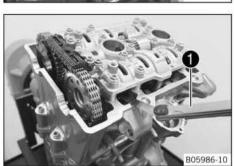
Check the valve clearance at the exhaust valves and the intake valves between the camshaft and cam lever using the special tool 1.
