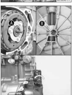
Position the clutch cover with the clutch cover gasket.
