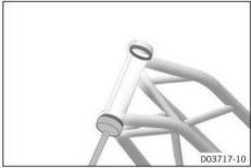
Press in the new bearing ring all the way using a suitable tool.
