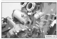
Grease the O-ring and mount the starter motor.
