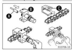
Mount press drift with the larger diameter in the spindle of the special tool. Turn the spindle counterclockwise.
