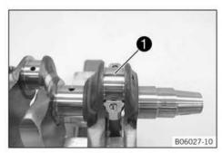
Position the bearing shells. Insert Plastigauge clearance gauge 1 90° offset to the bearing joint.
