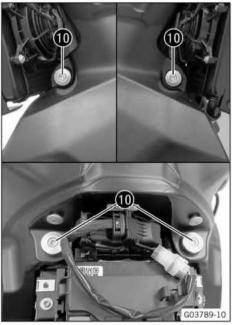
Remove screws **10** with bearing sleeves and rubber bushings.
