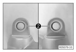
Remove seal rings 2 on both sides.
