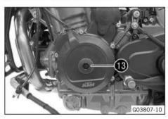
Remove screw plug 13 with the O-ring.
