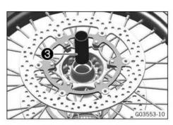
Clean, grease, and mount spacing tube 3.
