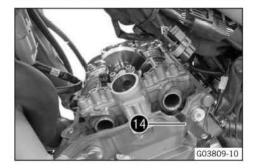
Check the valve clearance at the exhaust valves and the intake valves between the camshaft and cam lever using the special tool 14.
