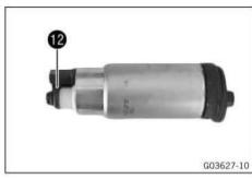
Remove O-ring 12 and mount new O-ring.
