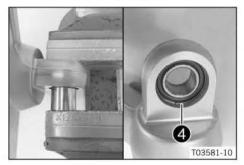
Push in the heim joint to the lock ring using the special tool.
