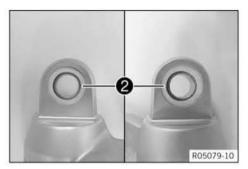
Mount and grease seal rings 2 on both sides.
