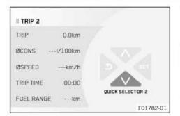
When the menu is closed, the **Quick Selector 2** display is opened by pressing the **DOWN** button.
