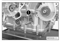
Position crankshaft to cylinder 1 TDC and lock with special tool 1.
