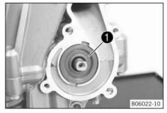
Grease and mount the new shaft seal ring 1.
