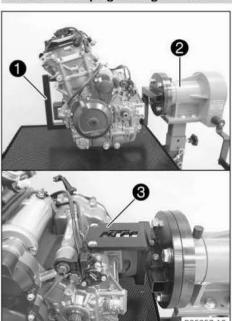
Mount special tool 1 on engine assembly stand 2.
