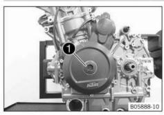
Remove screw of the alternator cover.
