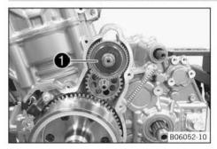
Take off torque limiter 1 with washer.
