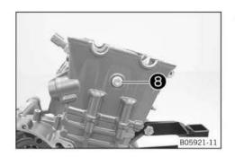
Mount and tighten screw 8 with gasket. Guideline
