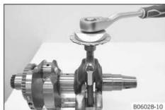
Position the conrod bearing cover. Mount and tighten the screws.
