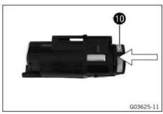
Mount new fuel filter 10 on the fuel pump.
