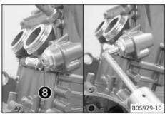
Remove screw 8 with the O-ring and use a special tool to push the timing chain tensioner toward the timing chain.
