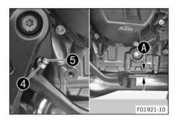
Loosen nut 4 and turn screw 5 correspondingly until the free travel A is present. If necessary, adjust the basic position of the foot brake lever.
