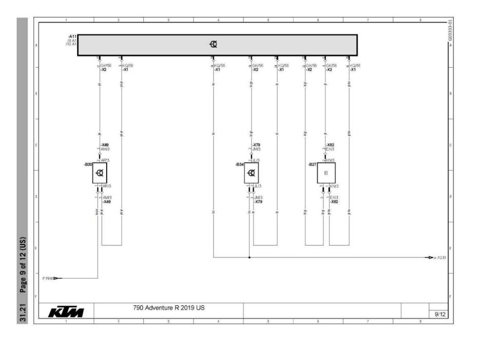
A11 Engine electronics control unit
