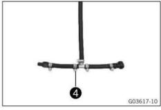
Mount special tool 6 and secure with a hose clip.
