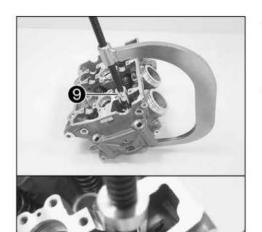
Tension valve spring with special tool 9.
