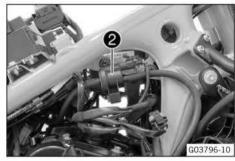
Position fuel evaporation valve 2 on the holder.
