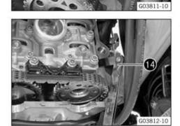
Check the valve clearance at the exhaust valves and the intake valves between the camshaft and cam lever using the special tool 14.
