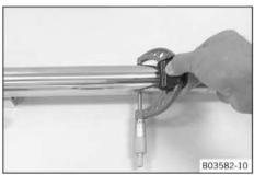
Measure the run-out of the inside fork tube.
