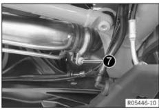
Position the clamp. Mount screw 7, but do not tighten yet.
