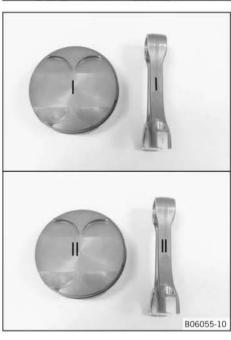
Mark the pistons and connecting rods belonging together correspondingly.
