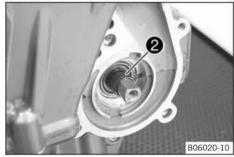
Remove water pump impeller 2.
