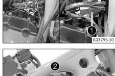
Pull fuel evaporation valve 2 off the holder and hang it to the side.
