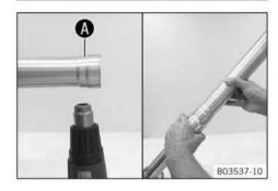
Warm up the outside fork tube in area of the lower sliding bushing.
