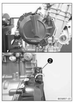
Swivel the clutch release lever 2 clockwise and take off clutch cover with clutch cover gasket.
