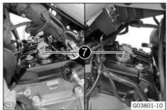
Mount and tighten the spark plugs using special tool 7.
