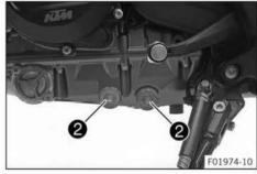
Remove oil drain plugs 2 with the magnets, O-rings, and oil screens.
