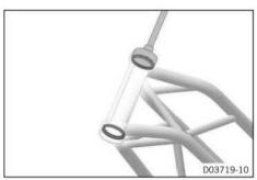
Press in the new bearing ring all the way using a suitable tool.
