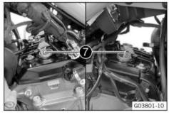
Remove spark plugs using special tool 7.
