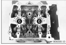
Remove shims 6 and label according to their normal built-in position.
