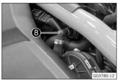
Thoroughly clean the plug-in connection of the fuel line using compressed air.
