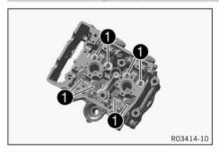
Check valve guides 1 using the special tool.
