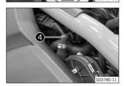
Thoroughly clean the plug-in connection of the fuel line using compressed air.
