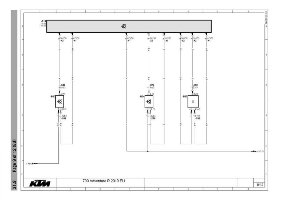
A11 Engine electronics control unit
