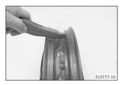
Carefully cut through the tubeless sealing profile and pull it off.
