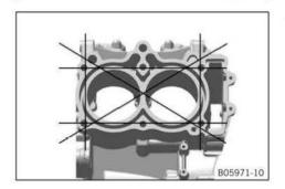
Using a straightedge and the special tool, check the sealing surface of the cylinder head for distortion.
