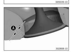
Check sealing seat A of the valves.
