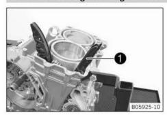
Remove the timing chain guide rail 1 from the top.
