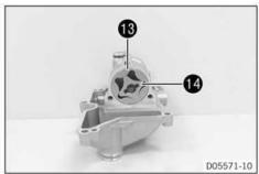
Remove external rotor 13 and internal rotor 14.
