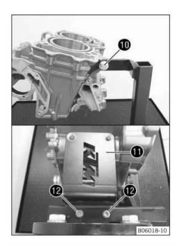
Position upper section of the engine case in the engine assembly stand, mount screw and tighten.
