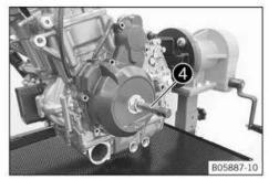
Mount special tool 4 and pull off the alternator cover.
