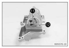
Remove pin and oil pump shaft .
