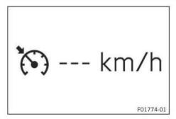
When cruise control is activated, the operating mode is shown on the combination instrument display.
