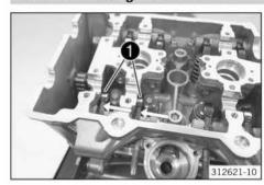
Push exhaust cam lever 1 on cylinder 2 to the side.
