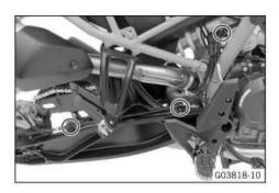
Secure the brake line and cable in the holders.
