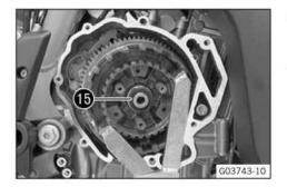
Hold the inner clutch hub with the special tool.
