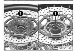
Grease new shaft seal rings and press them in until they are flush.
