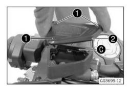
Correct the brake fluid to MAX marking ().
