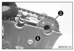
Pull up the timing chain and position the exhaust camshaft 2.
