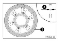
Check front and rear brake disc thickness at multiple points for the dimension **A**.
