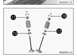
Remove valve spring retainers 11, valve springs, valve stem seals 12 and valve spring seats 13.
