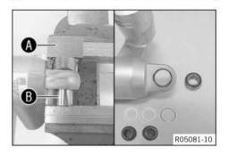
Place special tool (A) underneath and press out heim joint (3) using special tool B.
