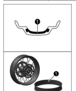
This vehicle uses a tubeless tire system in which a rim seal band **1** is used instead of the conventional tube.
