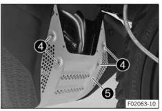
Remove screws 4 and engine guard 6.
