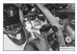
Pull off the throttle valve body toward the rear and remove to the side.
