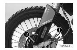
Position the fork protector. Mount screw ①, but do not tighten yet.
