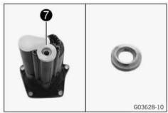
Position retaining waster 7 with the collar facing downward.
