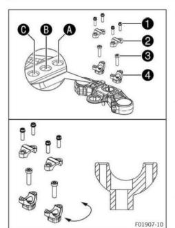
Remove screws **1**. Take off the handlebar clamps **2**. Position the handlebar so that screws **3** are accessible.
