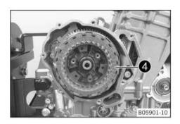
Remove clutch discs 4, support ring, and pretension ring.
