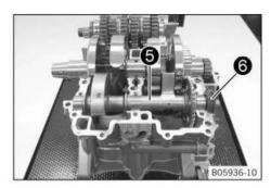
Remove balancer shaft 6 with shaft seal ring 6.
