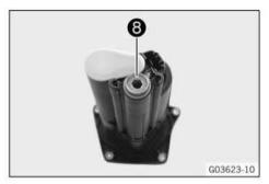
Mount pressure control valve 8 with new O-ring.
