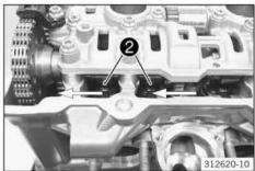
Push exhaust cam lever 2 on cylinder 2 to the side.
