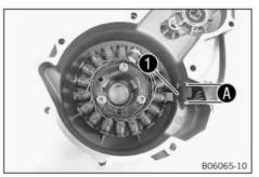
Apply sealing compound lightly in the area of the rubber grommet.
