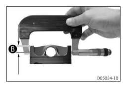
Measure the piston at the piston skirt, at right angles to the piston pin, at a distance B.
