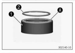
Before mounting, grease spacer 1 in area A and O-ring 2.
