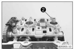
Remove the spark plugs using special tool 2.
