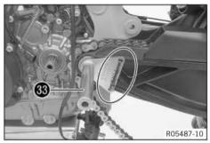
Mount special tool 33 and secure with a cable tie.
