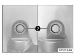
Remove seal rings 2 on both sides.
