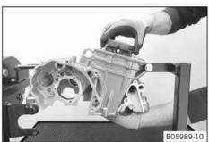
Remove piston with connecting rod upward out of the cylinder.
