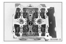
Mount and tighten screws 2.
