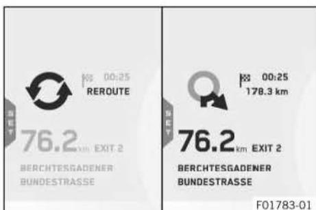
The **Navigation** display appears when the navigation function is active. In the **Navigation** display, the direction arrow, the distance from the destination, the estimated arrival time of the cellphone, the distance to the next waypoint and the street name are displayed. The **Navigation** display can be configured in the **Navigation** submenu.
