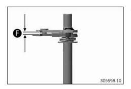
Check clearance **6** between the sliding plate and the shift quadrant.
