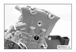
Mount and tighten screws 7.
