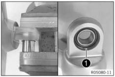
Press the heim joint against the lock ring using the special tool.
