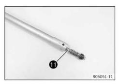
Slide piston rod into the cartridge.
