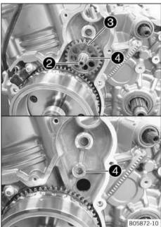
Take off shaft 2 and starter idler gear 3 with needle bearing and washers  $\Phi$ .
