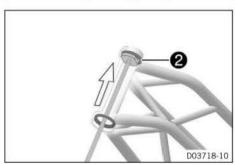
Remove upper bearing ring ② using a suitable tool.
