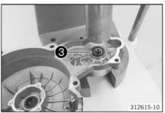
Press in new bearing 3 all the way using a suitable tool.
