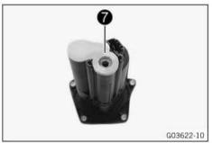
Remove pressure control valve 8 with O-ring.
