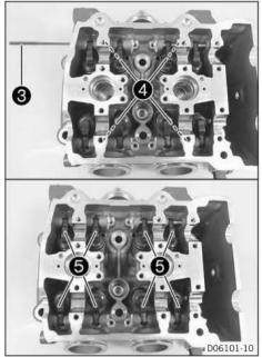
Mount disassembly tool M4 e.g. a spoke 3.
