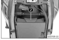
Remove air filter frame 3 with the air filter.
