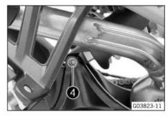
Tighten adjusting screw 4.
