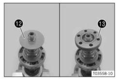
Mount shim stack 12 with the smaller washers facing downward.
