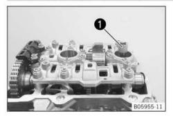
Mount and tighten the spark plugs using a special tool ①.
