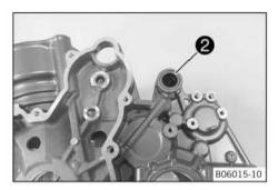
Remove shaft seal ring 2 of the shift shaft.
