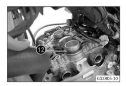
Grease the O-rings and mount spark plug shaft inserts
