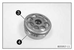
Turn the freewheel gear 3 counterclockwise and mount in the rotor 4.
