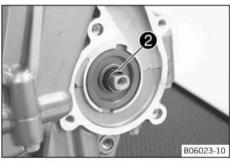
Mount the new water pump impeller 2.
