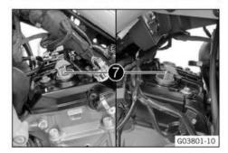
Remove spark plugs using special tool 7.
