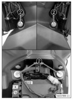
Mount and tighten screws 2 with the bearing sleeves and the rubber bushings.
