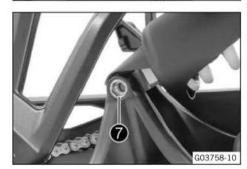
Loosen adjusting screw 7.
