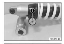
Clamp the shock absorber into the special tool.
