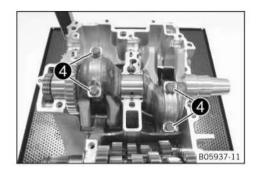
Mount and tighten new screws 4.
