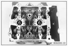
Place shims 6 into the valve spring retainer according to their normal built-in position.
