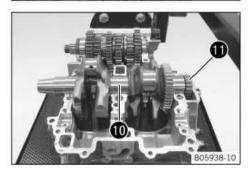
Remove crankshaft 10 with timing chain 11.
