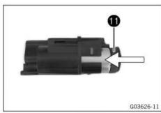
Mount fuel pump 1 in new fuel pump housing.
