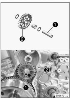
Mount shaft 1 and starter idler gear 2 with needle bearing and washers.
