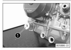
Tilt the motorcycle to one side and fill the oil filter housing to about ¼ full with engine oil.
