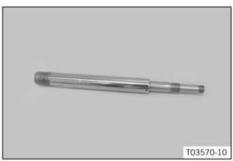
Measure the diameter of the piston rod.
