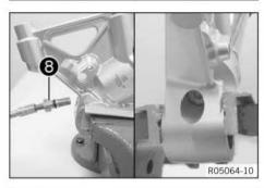
Mount screw 8 with the O-ring and tighten.
