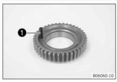
Mount dowel pin 1 in the primary gear wheel.
