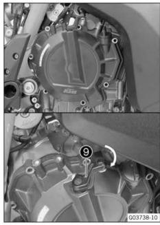
Swivel the clutch release lever 9 clockwise and take off clutch cover with clutch cover gasket.
