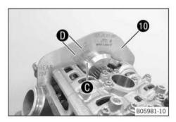
Check position of the balancer shaft with special tool 10.
