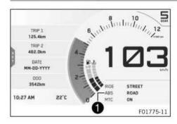
The ABS mode setting is shown in the **1** area of the display. The ABS can be configured in the **ABS** submenu.
