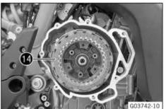
Remove clutch discs 14, support ring, and pretension ring.
