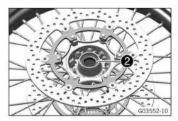
Using a suitable tool, press bearing 2 out from the inside to the outside.
