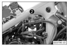
Position fuel evaporation valve 2 on the holder.
