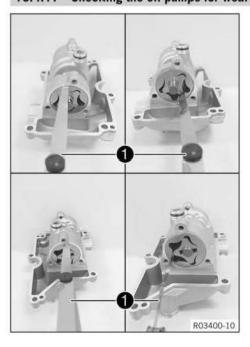
Use a feeler gauge **1** to measure the play between the external rotor and oil pump housing as well as between the external rotor and internal rotor.
