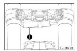
Steering damper article number  $\P$  is embossed on the underside of the steering damper.
