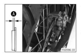
Check the brake linings for minimum thickness A.
