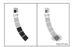
The fuel level display consists of bars. The more bars are lit, the more fuel is in the fuel tank.
