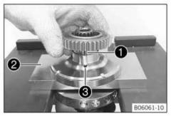
Position the crankshaft with special tool 2 in the press.
