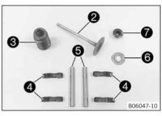
Check the valve stem diameter.
