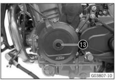
Mount and tighten screw plug 13 with the O-ring.
