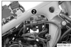
Pull fuel evaporation valve ② off the holder and hang it to the side.
