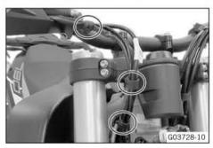
Route the cables without tension and secure with cable ties.
