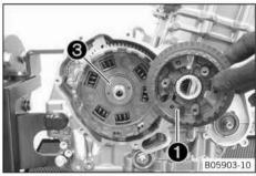
Take off inner clutch hub and washer and washer .
