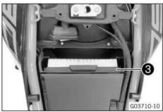
Remove air filter frame 3 with the air filter.
