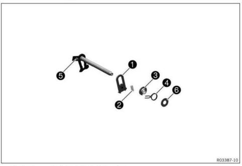
Fix the short end of the shift shaft in a vise.
