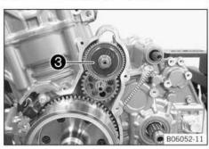
Mount torque limiter 3 with the rear washer.
