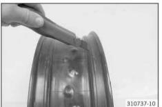
Carefully cut through the tubeless sealing profile and pull it off.
