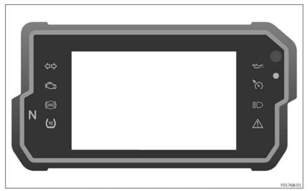
The indicator lamps offer additional information about the operating state of the motorcycle. When the ignition is switched on, all indicator lamps light up briefly, except for the TC indicator lamp ...
