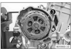
Remove clutch pressure cap 3.
