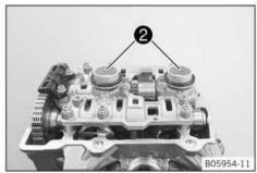
Grease the O-rings and mount spark plug shaft inserts **2** with gasket.
