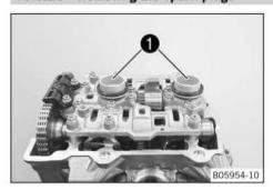
Remove spark plug shaft inserts 1 with the gaskets.
