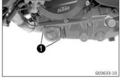
Position the special tool with the O-ring.
