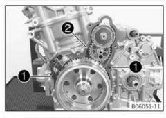
Apply sealing compound lightly in the area of the rubber grommet.
