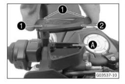
Correct the brake fluid to the MAX marking A.
