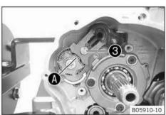
Twist shift drum until the neutral position (A) is aligned with the sliding plate (3).
