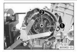
Hold the inner clutch hub with the special tool.
