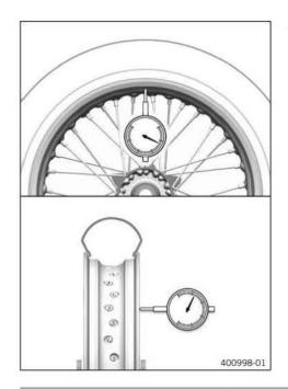
Check for lateral and radial run-out of the rims.
