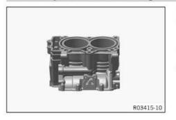
**Nikasil®** is a surface protection layer for a coating procedure developed by Mahle. The name is derived from the two materials used in this procedure - a layer of nickel into which is embedded the particularly hard silicone carbide.
