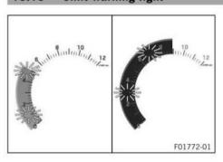
The shift warning light is integrated in the tachometer display. In the **Shift Light** submenu, the engine speed for the shift warning light can be set. The shift warning light is always active during the running-in phase (up to 1,000 km / 621 mi). The shift warning light can only be deactivated, and the values for **Lights up** and **Flashes** can only be adjusted after this. In **Lights up** the shift warning light flashes and in **Flashes** it flashes and the color changes.
