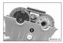
Turn the crankshaft counterclockwise by the specified value and set it to ignition top dead center of cylinder 1.
