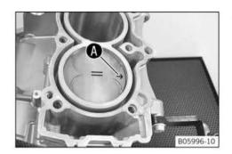
Ensure that piston marking A faces the exhaust side.
