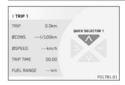
When the menu is closed, the **Quick Selector 1** display is opened by pressing the **UP** button.
