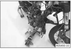
Turn engine and remove to the side.
