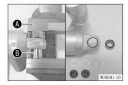
Place special tool **A** underneath and press out the heim joint with a special tool **B**.
