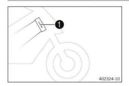
The vehicle identification number **1** is stamped on the right side of the steering head.
