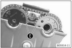
Turn the crankshaft counterclockwise by the specified value and set it to ignition top dead center of cylinder 2.
