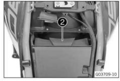
Remove air filter clamping wedge 2 upwards.
