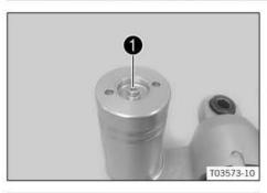
Mount screw with the O-ring and screw it in approx. 2 full turns, but do not tighten it fully yet.
