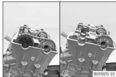
Raise the camshafts at the rear and take the timing chain off the rear sprocket. Remove the camshafts.
