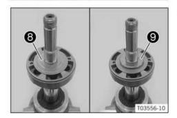
Mount rebound shim stack 8 with the smaller washers facing upward.
